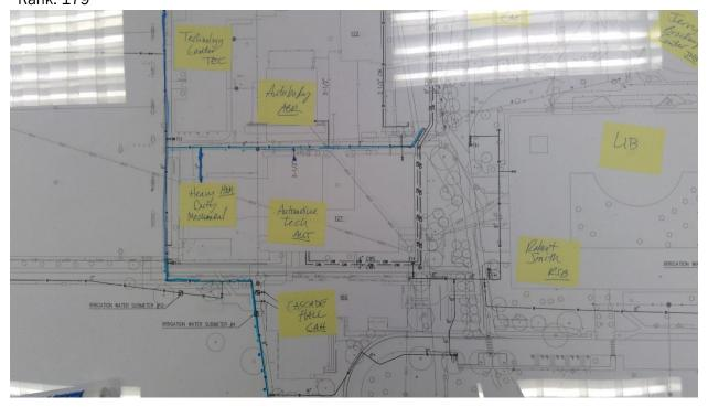
2601 South Seattle C. C. - Main Campus Potable Water Start location - Latitude: 47.5489017 Start location - Longitude: -122.3526055 End Location - Latitude: 47.5489669 End Location - Longitude: -122.352297 Depth: 4 Pipe Size: 2" Length: 100 Placement: Placement Method: Direct burried Material: Copper Under Hardscape: 1 Path Configuration: Multiple segments Placement Method: Direct burried Connections: 0 Age: 50 Expected life: 45 Survey Score: 4.2687488161079 Rank: 180
