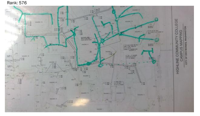
800 Highline C. C. - Main Campus Storm Start location - Latitude: 47.3878676 Start location - Longitude: -122.2993418 End Location - Latitude: 47.3875807 End Location - Longitude: -122.2994062 Depth: 4 Pipe Size: 6" Length: 250 Material: Transite Under Hardscape: 0.9 Path Configuration: Multiple segments Connections: 3 Age: 56 Expected life: 57 Survey Score: 3.76679840343442 Rank: 577
