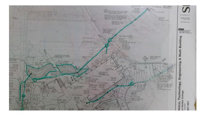
961 Grays Harbor College - Main Campus Storm Start location - Latitude: 46.9526835 Start location - Longitude: -123.8035265 End Location - Latitude: 46.9526993 End Location - Longitude: -123.8033937 Depth: 4 Pipe Size: 8" Length: 50 Material: Concrete Under Hardscape: 1 Path Configuration: Linear Connections: 1 Age: 66 Expected life: 52.61 Survey Score: 4.08623380562079
