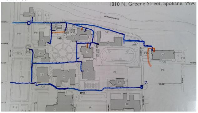
3864 Spokane C. C. - Main Campus Sewer Start location - Latitude: 47.6772517 Start location - Longitude: -117.3619061 End Location - Latitude: 47.6766081 End Location - Longitude: -117.3613431 Depth: 6 Pipe Size: 8" Length: 300 Material: Concrete Under Hardscape: 0.7 Path Configuration: Linear Connections: 0 Man holes: 2 Age: 52 Expected life: 57 Survey Score: 3.08881391668224 Rank: 656
