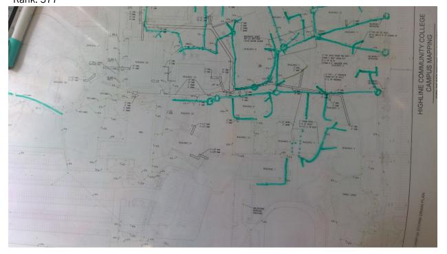
802 Highline C. C. - Main Campus Storm Start location - Latitude: 47.3875825 Start location - Longitude: -122.2993927 End Location - Latitude: 47.3876027 End Location - Longitude: -122.2997136 Depth: 4 Pipe Size: 8" Length: 100 Material: Transite Under Hardscape: 0.8 Path Configuration: Linear Connections: 0 Age: 56 Expected life: 57 Survey Score: 3.76679840343442 Rank: 578
