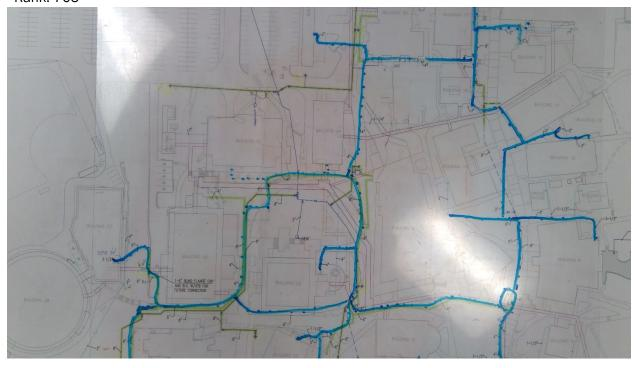
671 Highline C. C. - Main Campus Sewer Start location - Latitude: 47.387675 Start location - Longitude: -122.301093 End Location - Latitude: 47.387983 End Location - Longitude: -122.301094 Depth: 6 Pipe Size: 8" Length: 300 Material: Transite Under Hardscape: 1 Path Configuration: Linear Connections: 1 Man holes: 0 Age: 54 Expected life: 57 Survey Score: 2.96679840343442 Rank: 706
