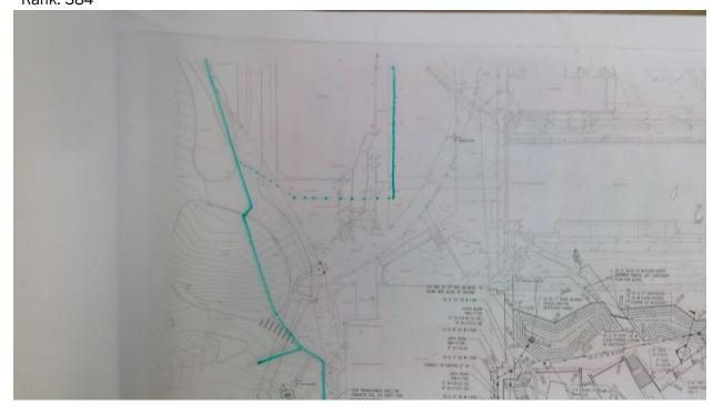
967 Grays Harbor College - Main Campus Sewer Start location - Latitude: 46.9526581 Start location - Longitude: -123.8007487 End Location - Latitude: 46.9529009 End Location - Longitude: -123.801175 Depth: 12 Pipe Size: 6" Length: 150 Material: Transite Under Hardscape: 0.9 Path Configuration: Linear Connections: 0 Man holes: 1 Age: 50 Expected life: 52.61 Survey Score: 2.08623380562079 Rank: 1951
