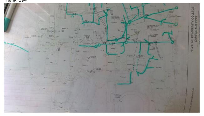
802 Highline C. C. - Main Campus Storm Start location - Latitude: 47.3875825 Start location - Longitude: -122.2993927 End Location - Latitude: 47.3876027 End Location - Longitude: -122.2997136 Depth: 4 Pipe Size: 8" Length: 100 Material: Transite Under Hardscape: 0.8 Path Configuration: Linear Connections: 0 Age: 56 Expected life: 57 Survey Score: 4.16679840343442 Rank: 195
