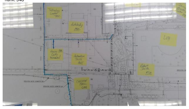
2601 South Seattle C. C. - Main Campus Potable Water Start location - Latitude: 47.5489017 Start location - Longitude: -122.3526055 End Location - Latitude: 47.5489669 End Location - Longitude: -122.352297 Depth: 4 Pipe Size: 2" Length: 100 Placement: Placement Method: Direct burried Material: Copper Under Hardscape: 1 Path Configuration: Multiple segments Placement Method: Direct burried Connections: 0 Age: 50 Expected life: 45 Survey Score: 3.8687488161079 Rank: 549
