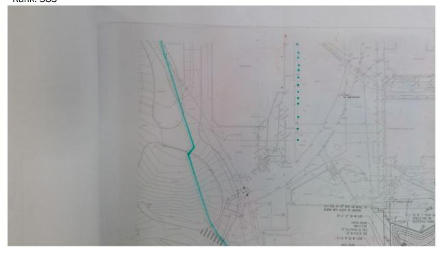
965 Grays Harbor College - Main Campus Storm Start location - Latitude: 46.9530929 Start location - Longitude: -123.8030085 End Location - Latitude: 46.9531447 End Location - Longitude: -123.8036743 Depth: 4 Pipe Size: 8" Length: 150 Material: Concrete Under Hardscape: 0.5 Path Configuration: Multiple segments Connections: 2 Age: 54 Expected life: 52.61 Survey Score: 3.68623380562079 Rank: 384
