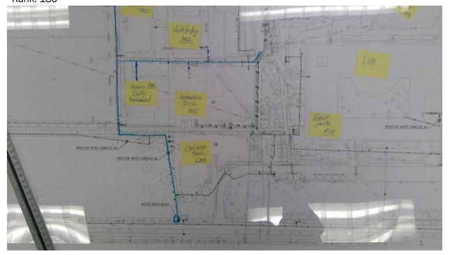
2614 South Seattle C. C. - Main Campus Potable Water Start location - Latitude: 47.5485203 Start location - Longitude: -122.3526487 End Location - Latitude: 47.5486698 End Location - Longitude: -122.3515766 Depth: 4 Pipe Size: 3" Length: 300 Placement: Placement Method: Direct burried Material: Copper Under Hardscape: 1 Path Configuration: Multiple segments Placement Method: Direct burried Connections: 2 Age: 44 Expected life: 45 Survey Score: 3.0687488161079 Rank: 664
