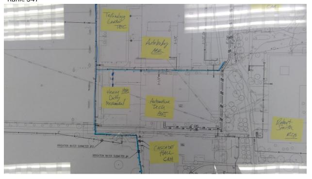
2600 South Seattle C. C. - Main Campus Potable Water Start location - Latitude: 47.5490906 Start location - Longitude: -122.3525629 End Location - Latitude: 47.5490254 End Location - Longitude: -122.3526889 Depth: 4 Pipe Size: 2" Length: 50 Placement: Placement Method: Direct burried Material: Copper Under Hardscape: 1 Path Configuration: Linear Placement Method: Direct burried Connections: 0 Age: 50 Expected life: 45 Survey Score: 3.8687488161079 Rank: 548
