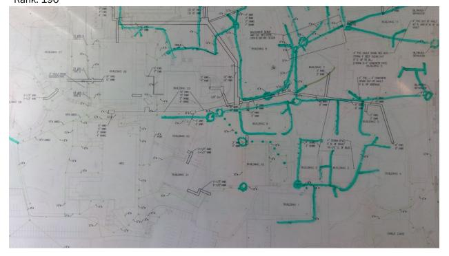
807 Highline C. C. - Main Campus Storm Start location - Latitude: 47.3877207 Start location - Longitude: -122.2997484 End Location - Latitude: 47.3877788 End Location - Longitude: -122.2998128 Depth: 4 Pipe Size: 6" Length: 50 Material: Transite Under Hardscape: 0.2 Path Configuration: Multiple segments Connections: 2 Age: 56 Expected life: 57 Survey Score: 2.56679840343442 Rank: 1282
