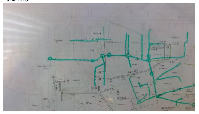
777 Highline C. C. - Main Campus Storm Start location - Latitude: 47.3886464 Start location - Longitude: -122.2998183 End Location - Latitude: 47.3882435 End Location - Longitude: -122.2998088 Depth: 4 Pipe Size: 12" Length: 150 Material: Concrete Under Hardscape: 0.7 Path Configuration: Multiple segments Connections: 1 Age: 54 Expected life: 57 Survey Score: 3.76679840343442
