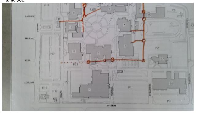
3909 Spokane C. C. - Main Campus Sewer Start location - Latitude: 47.6732927 Start location - Longitude: -117.3614385 End Location - Latitude: 47.6732984 End Location - Longitude: -117.3606298 Depth: 8 Pipe Size: 8" Length: 200 Material: Clay Under Hardscape: 1 Path Configuration: Linear Connections: 1 Man holes: 1 Age: 52 Expected life: 46.75 Survey Score: 4.28881391668224 Rank: 161
