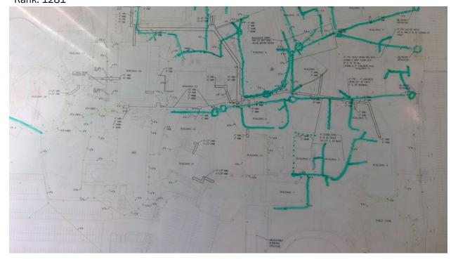
806 Highline C. C. - Main Campus Storm Start location - Latitude: 47.3877699 Start location - Longitude: -122.2998817 End Location - Latitude: 47.388112 End Location - Longitude: -122.3006096 Depth: 6 Pipe Size: 10" Length: 250 Material: Concrete Under Hardscape: 0.1 Path Configuration: Multiple segments Connections: 2 Age: 56 Expected life: 57 Survey Score: 4.16679840343442 Rank: 196
