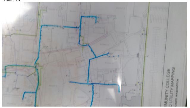
664 Highline C. C. - Main Campus Potable Water Start location - Latitude: 47.389753 Start location - Longitude: -122.299866 End Location - Latitude: 47.389753 End Location - Longitude: -122.299866 Depth: 4 Pipe Size: 2" Length: 100 Placement: Placement Method: Direct burried Material: Copper Under Hardscape: 1 Path Configuration: Multiple segments Placement Method: Direct burried Connections: 2 Age: 54 Expected life: 45 Survey Score: 4.56679840343442 Rank: 235
