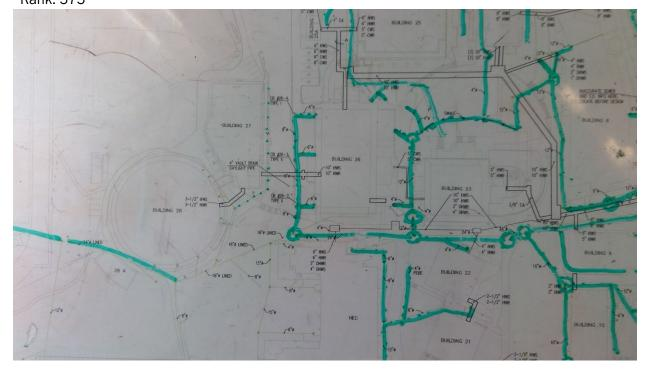
836 Highline C. C. - Main Campus Storm Start location - Latitude: 47.3884216 Start location - Longitude: -122.3026907 End Location - Latitude: 47.38822 End Location - Longitude: -122.3024467 Depth: 4 Pipe Size: 6" Length: 100 Material: Transite Under Hardscape: 0.4 Path Configuration: Linear Connections: 2 Age: 56 Expected life: 57 Survey Score: 3.36679840343442 Rank: 576
