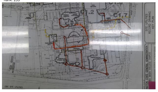
3522 Columbia Basin College - Main Campus Sewer Start location - Latitude: 46.2510462 Start location - Longitude: -119.1219423 End Location - Latitude: 46.2510977 End Location - Longitude: -119.1214092 Depth: 6 Pipe Size: 6" Length: 150 Material: Clay Under Hardscape: 0.2 Path Configuration: Linear Connections: 1 Man holes: 1 Age: 62 Expected life: 46.75 Survey Score: 5.12514950212143 Rank: 154
