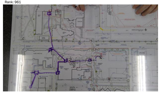
Yakima Valley C. C. - Main Campus Communication Start location - Latitude: 46.5848547 Start location - Longitude: -120.5278182 End Location - Latitude: 46.5844316 End Location - Longitude: -120.5277156 Depth: 2 Length: 150 Placement: Placement Method: Buried Conduit Fiber Size: Unknown Under Hardscape: 0.9 Path Configuration: Multiple segments Placement Method: Buried Conduit Conduit Size: 4" Number Of Conduits: 4 Age: 56 Expected life: 60 Survey Score: 2.8
