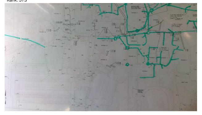
809 Highline C. C. - Main Campus Storm Start location - Latitude: 47.387601 Start location - Longitude: -122.2997449 End Location - Latitude: 47.3875919 End Location - Longitude: -122.3004048 Depth: 6 Pipe Size: 10" Length: 100 Material: Concrete Under Hardscape: 0.2 Path Configuration: Linear Connections: 0 Age: 56 Expected life: 57 Survey Score: 4.16679840343442 Rank: 197
