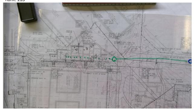
2291 Everett C. C. - Main Campus Sewer Start location - Latitude: 48.0061441 Start location - Longitude: -122.2037722 End Location - Latitude: 48.0061555 End Location - Longitude: -122.203251 Depth: 14 Pipe Size: 8" Length: 200 Material: PVC Under Hardscape: 1 Path Configuration: Linear Connections: 0 Man holes: 2 Age: 66 Expected life: 63 Survey Score: 5.20858230814294 Rank: 114
