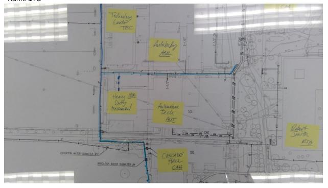
2600 South Seattle C. C. - Main Campus Potable Water Start location - Latitude: 47.5490906 Start location - Longitude: -122.3525629 End Location - Latitude: 47.5490254 End Location - Longitude: -122.3526889 Depth: 4 Pipe Size: 2" Length: 50 Placement: Placement Method: Direct burried Material: Copper Under Hardscape: 1 Path Configuration: Linear Placement Method: Direct burried Connections: 0 Age: 50 Expected life: 45 Survey Score: 4.2687488161079 Rank: 179
