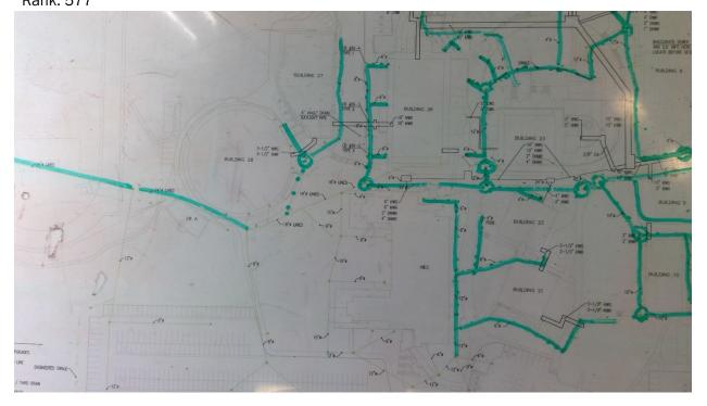
857 Highline C. C. - Main Campus Storm Start location - Latitude: 47.3868007 Start location - Longitude: -122.3015691 End Location - Latitude: 47.3868364 End Location - Longitude: -122.3018944 Depth: 4 Pipe Size: 6" Length: 100 Material: Transite Under Hardscape: 1 Path Configuration: Multiple segments Connections: 3 Age: 56 Expected life: 57 Survey Score: 4.16679840343442 Rank: 199
