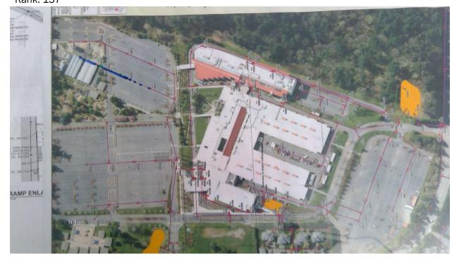
1930 Lake Washington I. T. - Main Campus Storm Start location - Latitude: 47.7040745 Start location - Longitude: -122.1656912 End Location - Latitude: 47.7040258 End Location - Longitude: -122.1651118 Depth: 2 Pipe Size: 15" Length: 200 Material: CMP Under Hardscape: 0.8 Path Configuration: Multiple segments Connections: 3 Age: 38 Expected life: 19.1 Survey Score: 4.28912953582136 Rank: 158
