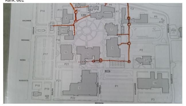
3900 Spokane C. C. - Main Campus Sewer Start location - Latitude: 47.6736358 Start location - Longitude: -117.3608109 End Location - Latitude: 47.6736636 End Location - Longitude: -117.3622801 Depth: 10 Pipe Size: 8" Length: 400 Material: Concrete Under Hardscape: 0.1 Path Configuration: Linear Connections: 1 Man holes: 2 Age: 52 Expected life: 57 Survey Score: 3.08881391668224 Rank: 662
