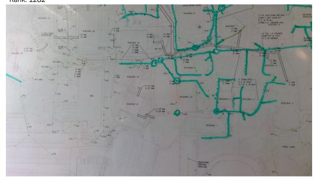
808 Highline C. C. - Main Campus Storm Start location - Latitude: 47.387641 Start location - Longitude: -122.299879 End Location - Latitude: 47.3877881 End Location - Longitude: -122.2998442 Depth: 4 Pipe Size: 6" Length: 100 Material: Transite Under Hardscape: 0 Path Configuration: Multiple segments Connections: 2 Age: 56 Expected life: 57 Survey Score: 3.36679840343442 Rank: 573
